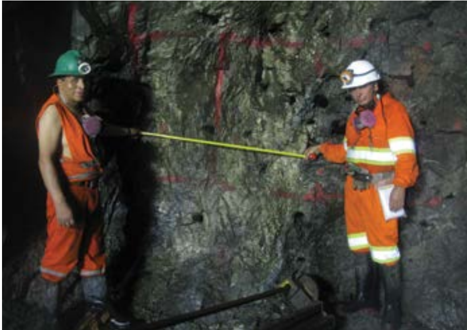
Left – High grade chalcopyrite vein over a width of 1.2 metres
