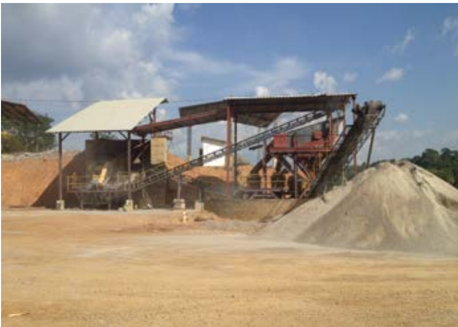
Left – Primary crushing plant producing crushed ore for processing
